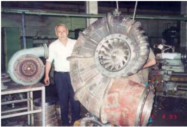
Fig. 10.9. Francis type turbine manufactured in Armenia by Vorotan LLC
