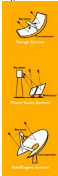
◀ Fig. 4.1. The schemes of operation of solar thermal power technologies
